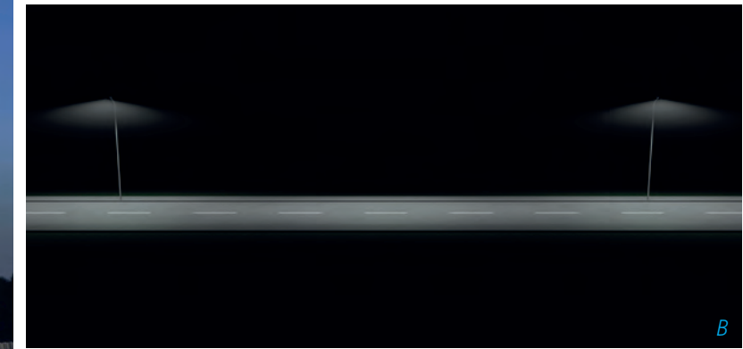
Figure 19B An installation using luminaires with high performance optics that emit light laterally over a large distance, ensuring that the road is evenly illuminated and visual acuity maintained
